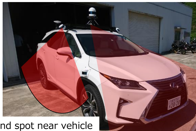
Monitoring in front of vehicle ( Nonmechanical PCSEL-LiDAR)
