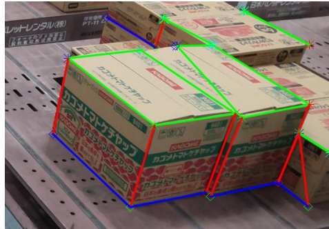
Detects boxes from pallet packing
