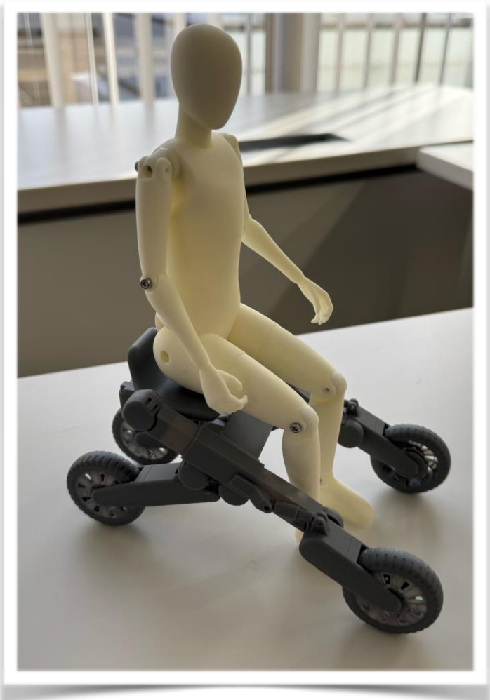
1/6 scale rapid prototyping model and transformation function verification prototype
