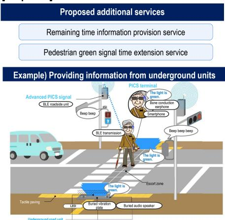
In addition to verification of services for people with visual impairments, also verify services for use of traffic signal information by devices other than mobile phones, such as autonomous delivery robots (including making improvements to existing apps and providing information to vehicles)
