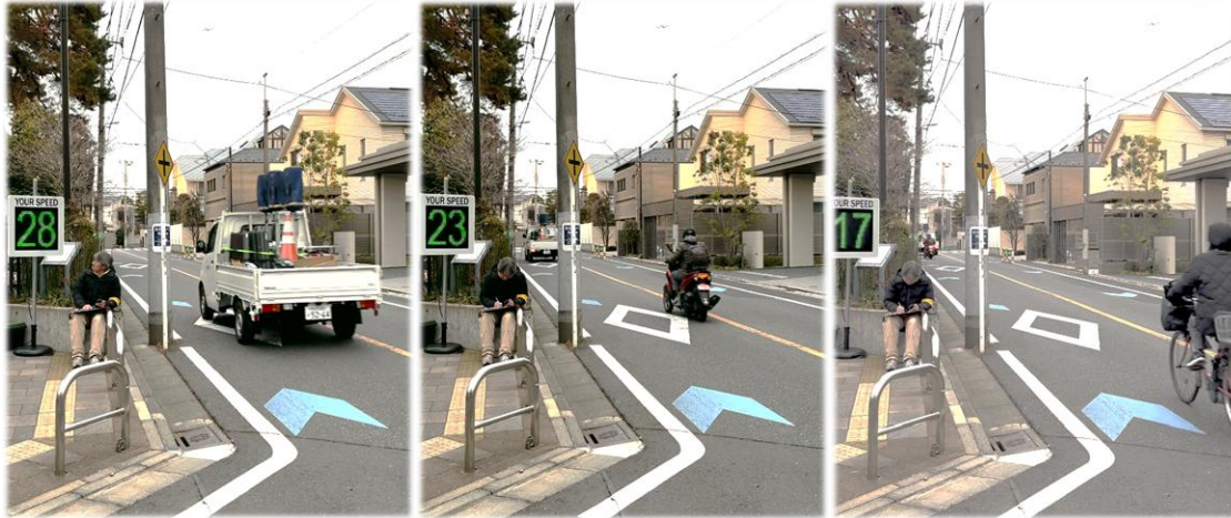
The speed-measurement display detecting and measuring various vehicles
