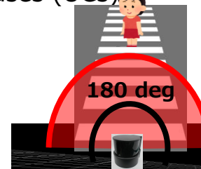
Pedestrian remaining unobservable due to falling into layer gaps (VLP-16)
