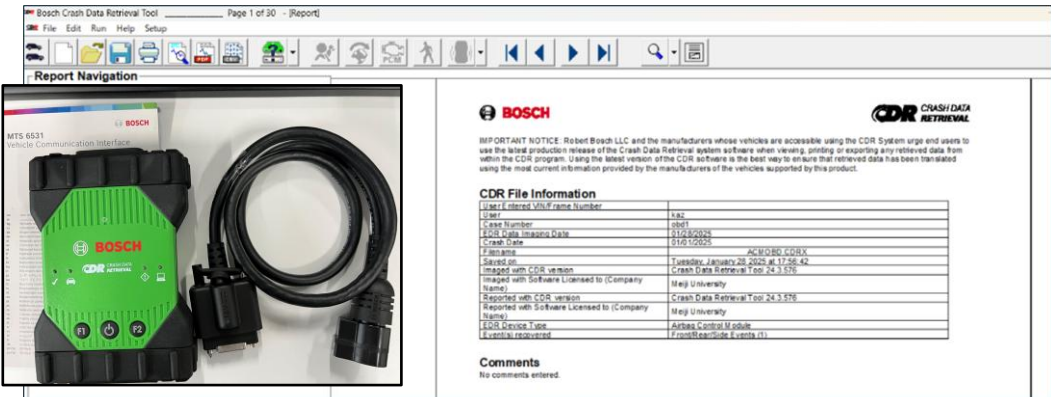
Fig. 2. Actual CDR operation and CDR equipment (Toyota vehicle)
