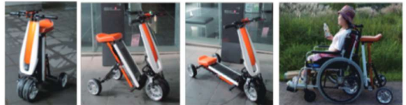
Walker (-2km/h) Mobility Scooter (Max 6km/h) Kick Skater (Max 10km/h, Make Energy) Wheel chair with multi-purpose mobility for power-assist
